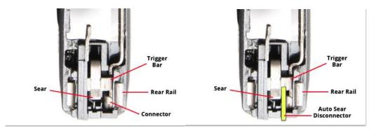
Images showing the back end of a Glock pistol with and without an auto sear disconnector
