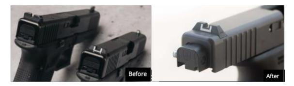
39. The auto sear has a small protrusion called a "disconnector" that, once installed, pushes the pistol's internal trigger bar down, allowing the striker to continue firing as the slide reciprocates with recoil. The ability to fire continuously, without the shooter having to pull and release the trigger repeatedly, allows for a much faster rate of fire.
